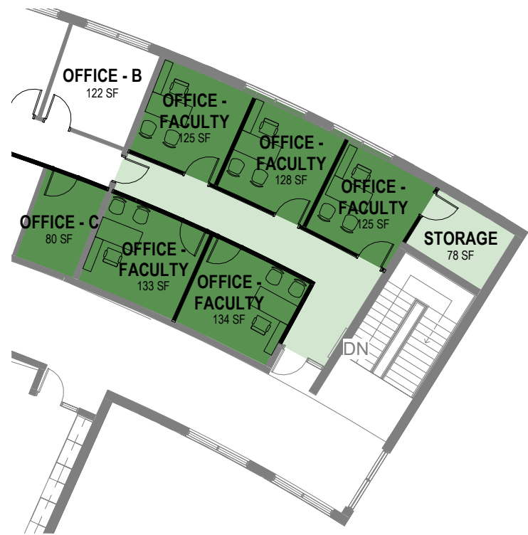
1 *SECOND LEVEL - RENOVATION - OFFICE SCALE: 1/16" = 1'-0"
